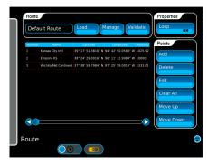
Routes with up to 10,000 route points, may be saved and recalled under a user entered route name, using the route file management system.
